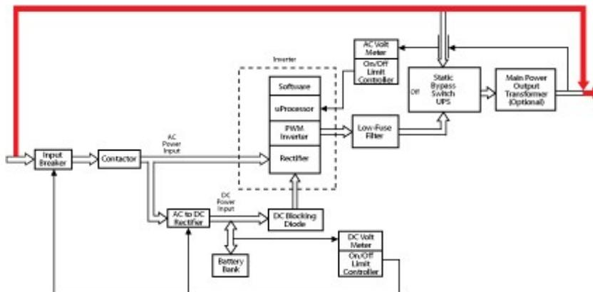
Figure 4 Single Line Drawings –External Maintenance Bypass Operation
