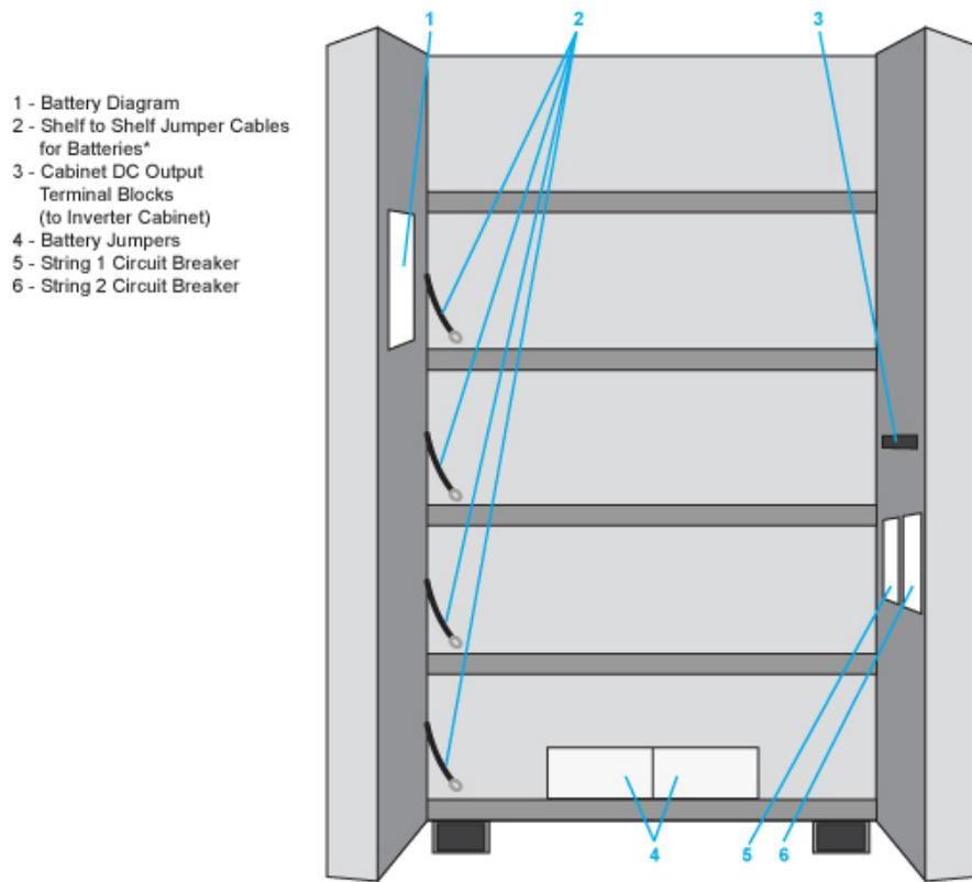
Note: Wires from battery cabinet to inverter to be provided by others.
