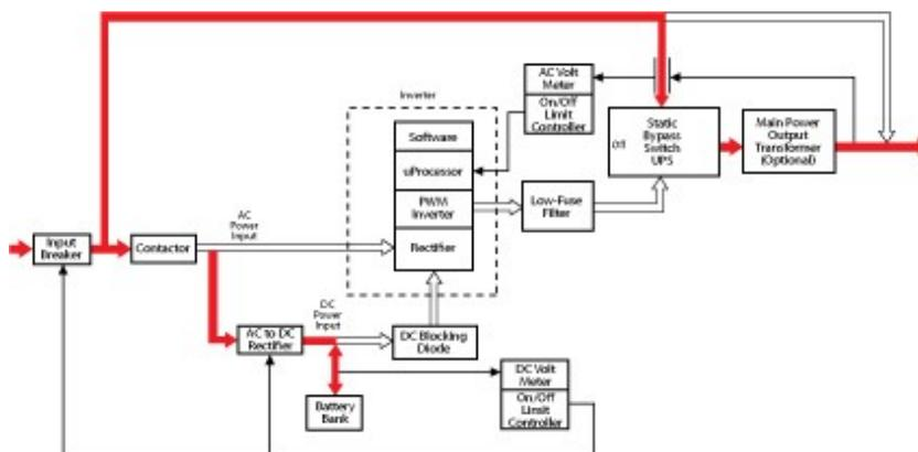
Figure 2 Single Line Drawing - Static Bypass Operation
